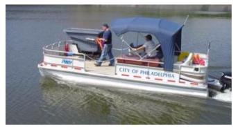
That's the smaller skimmer. It doesn't have a name. They have two such watercraft; the larger is called the R.E. Ro, which operates in the tidal reaches of the Schuylkill and the Delaware, for a total of 32 river miles. The smaller boat operates in the non-tidal part of the Schuylkill, north of the Fairmount Dam
