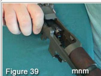
Cycle bolt as shown in **Figures 39 and 40** and make sure it moves easily without any binding or stoppage.
