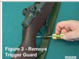
Use the slotted screwdriver to pull trigger housing guard to rear and then downward.
