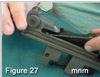
Turn receiver over and insert bolt into receiver as shown in **Figure 27**.
