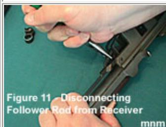
With receiver bottom facing up, use the needle nose pliers and disconnect the follower rod from the follower arm in the receiver.
