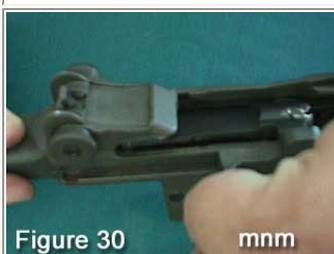
Then pull operating rod forward catching the bolt and locking into place.
