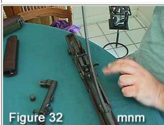
Reinstall operating rod spring by sliding the open spring end into the operating rod as shown in **Figure 32**.
