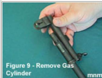
Carefully remove gas cylinder from rifle barrel and gas piston.
