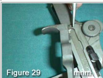
To attach operating rod, begin by taking lug of operating rod and inserting it into the channel at rear of receiver as shown in **Figure 29**.
