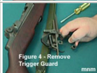
Remove the trigger assembly by grasping trigger guard and pulling down and away from the rifle.
