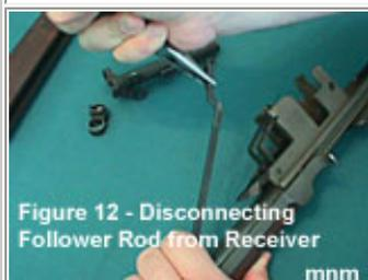
Once the follower arm is disconnected from follower arm, remove the follower rod and spring by pulling out of operating rod.
