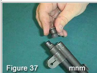
Hand thread into gas cylinder as shown in **Figure 37**.
