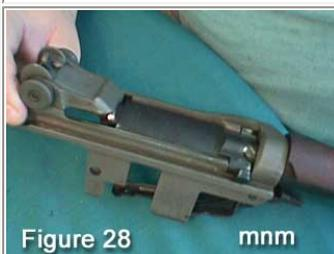
**Figure 28** shows the bolt properly installed into the receiver.
