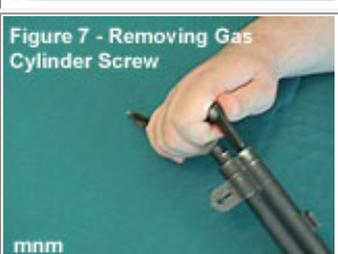
Using the slotted screwdriver attachment on the Garand Tool, unscrew the gas cylinder screw at the end of the gas cylinder. The use of the Garand Tool is recommended to do this task because of the size of the slots in the end of the screw would require a very large slotted screwdriver, which most people don't have on hand. Also the handle can be turned to a right angle to the screw driver, which gives considerably more torque than a normal screwdriver.
