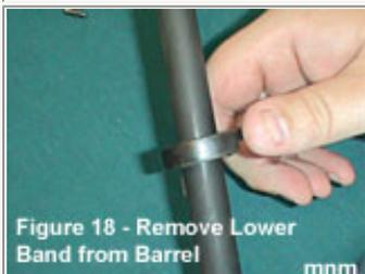
Slide lower band from barrel and set aside.
