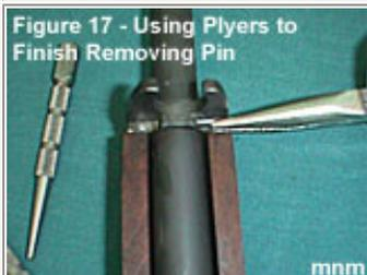
Using the needle nose pliers - finish removing retaining Pin.
