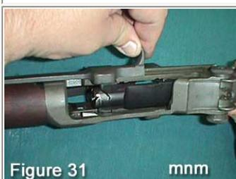
Test whether bolt and operating rod are properly installed by lightly cycling back and forth to make sure there is no binding or stoppage as shown in **Figure 31**.
