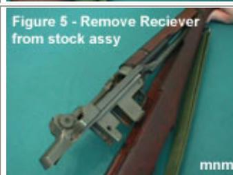
Remove receiver and barrel from stock by pulling up and away from stock.
