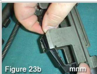
After bullet guide is in place, insert follower with shoulders in grooves in receiver. Insert follower arm, tilt until lugs pass through bullet guide. Insert operating rod catch and then insert pin as shown in **Figure 23b**.
