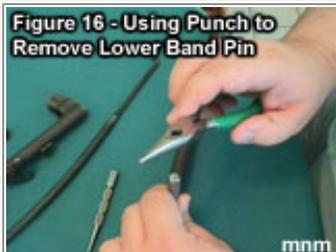
Use the medium punch to tap pin out of lower band, you may have to use the small punch to finish guiding pin out of band.
