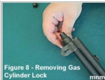
Finish unscrewing the gas cylinder lock using your hand.
