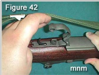
Turn rifle over and the trigger assembly into receiver by carefully aligning lugs in the trigger assembly in the channels in the receiver. Snap Trigger guard down and lock into place.
