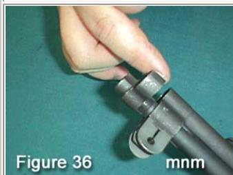
Hand thread gas cylinder lock over end threads on barrel end as shown in **Figure 36**. Screw it onto barrel until it is flush then back it off until it is aligned for insertion of gas lock screw.
