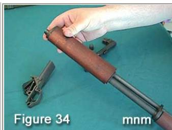
Slide the front hand guard over barrel and piston as shown in **Figure 34**.
