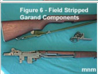
Displayed in **Figure 6**, is the M1 Garand field stripped into its three main parts: 1) receiver and barrel assembly, 2) stock, and 3) the trigger assembly.
