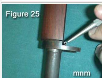
Insert pin into lower band and tap into hole as shown in **Figure 25**.
