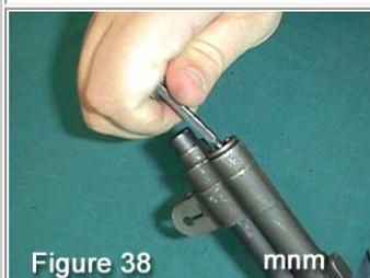
Take Garand Tool and tighten the gas cylinder screw until fairly tight as shown in **Figure 38**.
