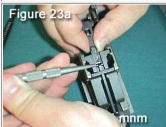
Now place the bullet guide in place as shown in **Figure 23a** .
