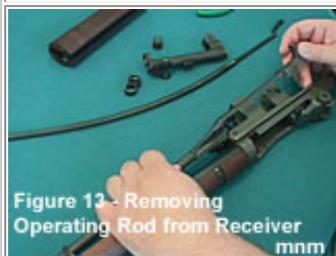
While holding the operating rod handle, pull back to rear of receiver, then pull up and then forward.
