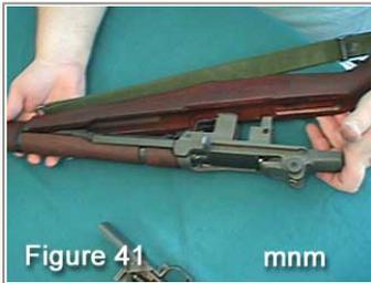
Insert receiver and barrel assembly into stock as shown in **Figure 41**.
