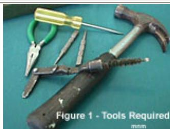
To properly disassemble an M1 Garand you need a slotted screw driver, a needle nose pliers, a small punch, a medium punch, and an M1 Garand Original Combination Maintenance Tool.
