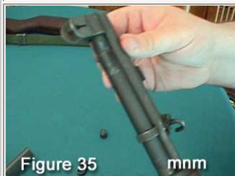
Slide gas cylinder over barrel and piston as shown in **Figure 35**.
