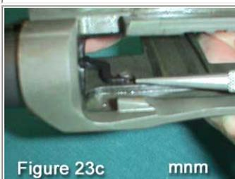
Look inside receiver and make sure the catch operating arm is as shown in **Figure 23c**.
