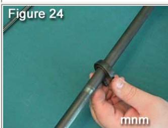
After sliding the rear hand guard over the barrel and to the front of the receiver, slide the lower band over barrel and up against rear hand guard.
