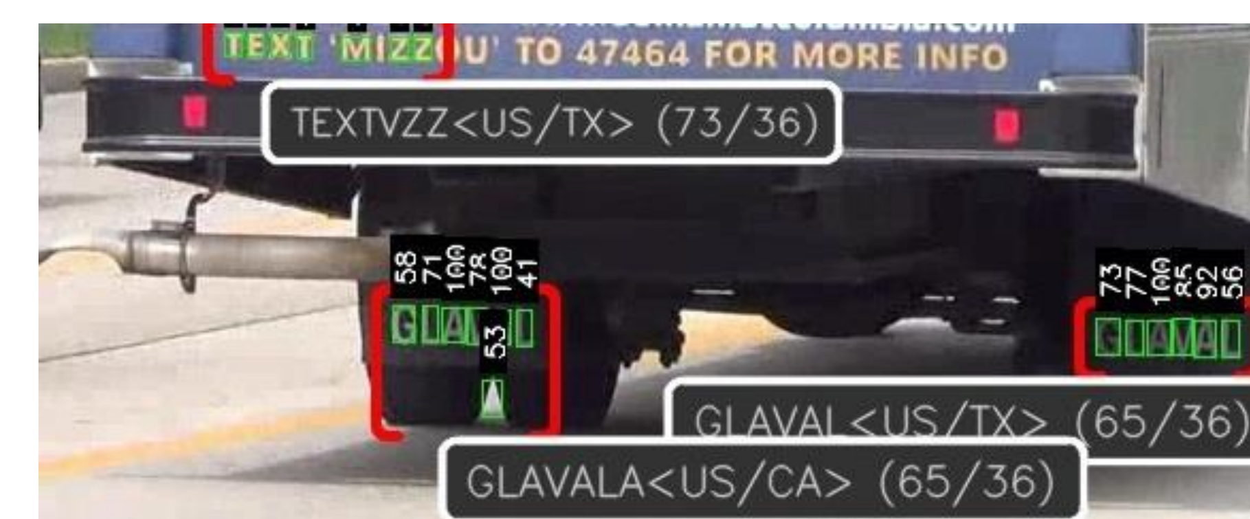
Figure 7. Example of Texts on a Bus Body (Vision Components, ANPR Demo Software).
