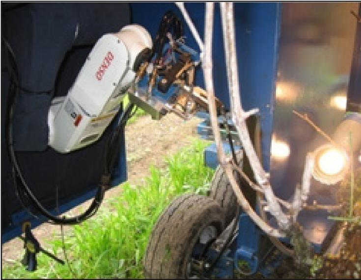
**Figure 4-** Robotic arm with attached customized pruner.
