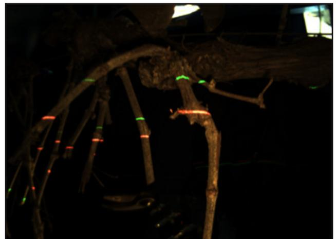
**Figure 5-** View from a pruner camera during cutting. The image is "upside down" as this orientation often affords better cutting positions. Red and green lasers are used to help guide the pruner to the cut point.
