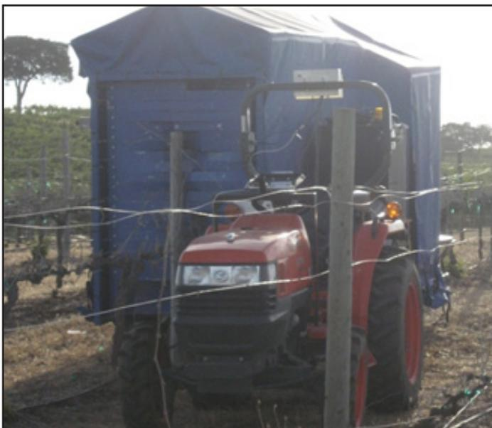
Figure 1- The Vision Robotics autonomous grapevine pruner.
