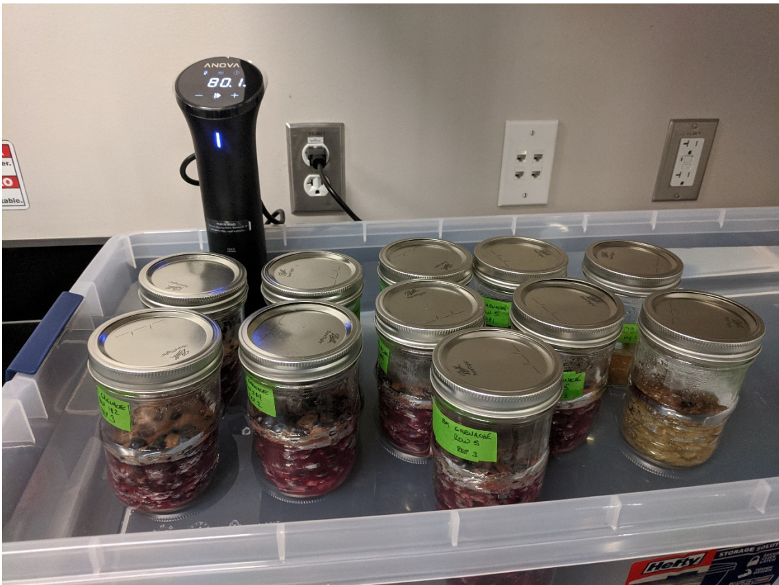
Figure 1 Under-the-bed storage box set up as a nano-scale fermentation water bath, with sous vide machine for temperature control. These are 16 oz. canning jars, with lids and bands loosely applied to allow CO 2 to escape.
