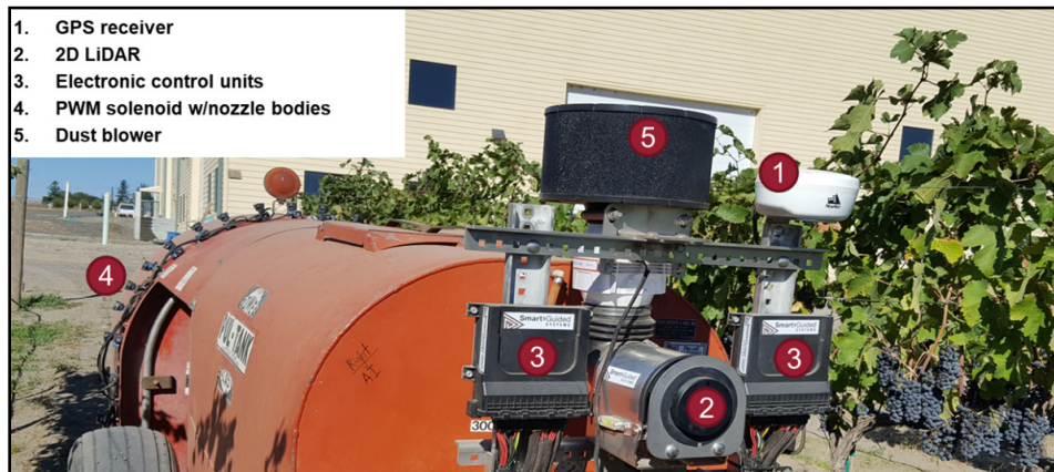
Fig. 1 - Intelligent sprayer retrofit system installed on a Rears airblast sprayer.
