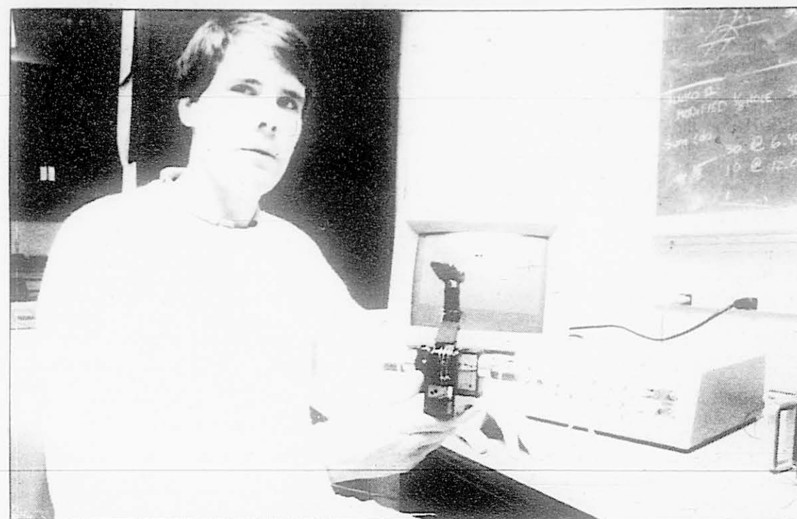
Scott Leaver, a mechanical engineer, displays a mechanical finger which can actually "feel." It can sense the size and weight of such objects as an egg, and may be a precursor to robotic hands.
