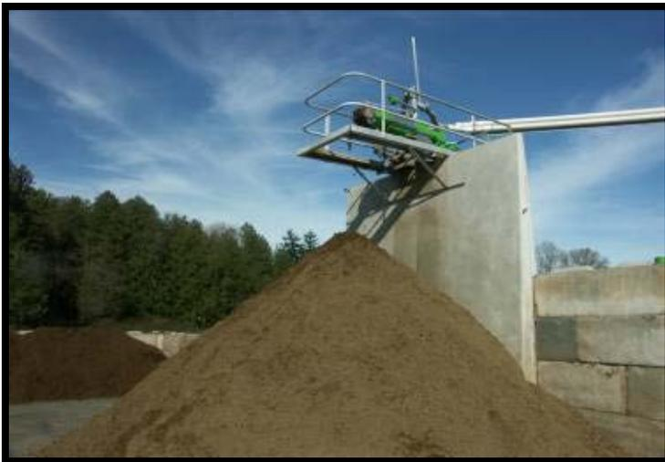
Figure 4.1: Fibrous product after AD and mechanical separation
