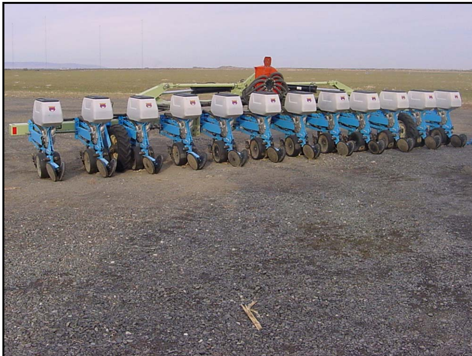
Williamson farm—planter, attached behind strip-tiller when in use.
