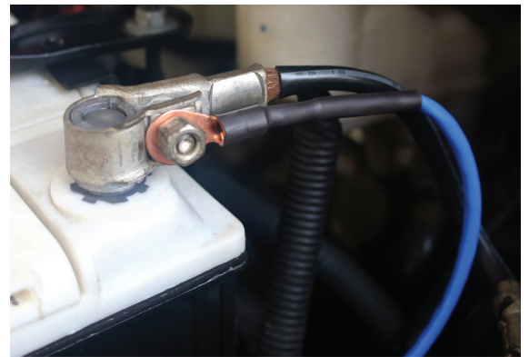
Typical Installation on Lead Acid Battery
