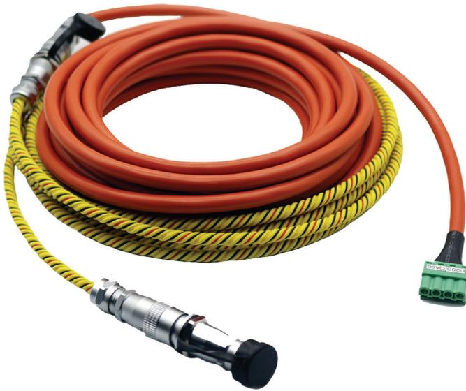
The rope water sensor comes in two parts, the orange non-sensing cable, and the yellow sensing cable. IP66 rated waterproof connectors join the two sections of rope together, with an additional connector at the tail end allowing the sensor to be extended with additional lengths as required. Lay these rope water sensors out around the perimeter of your room, or underneath aisles in your data center to give early warning of potential water leaks and avoid costly damage.
