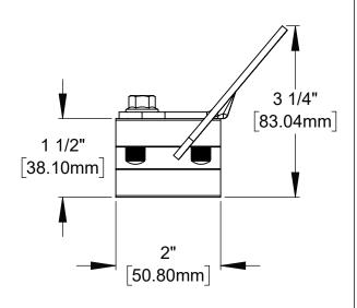
NOTE: SINGLE LOCK SEAMS MUST HAVE A HORIZONTAL LEG MEASUREMENT OF 5/8" OR GREATER FOR CLAMP TO ATTACH
