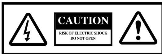
**CAUTION!** To reduce the risk of electric shock and fire, do not remove the cover or back plate of this device. There are no user serviceable parts inside. Please refer all servicing to licensed service technicians. Avis: Risque de choc électrique, ne pas ouvrir.
