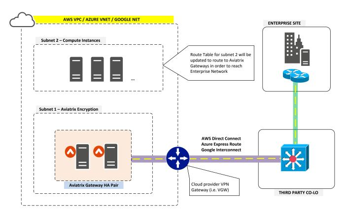
In the diagram above, an encrypted IPSec tunnel is established between the Aviatrix gateway and the customer's edge router.
