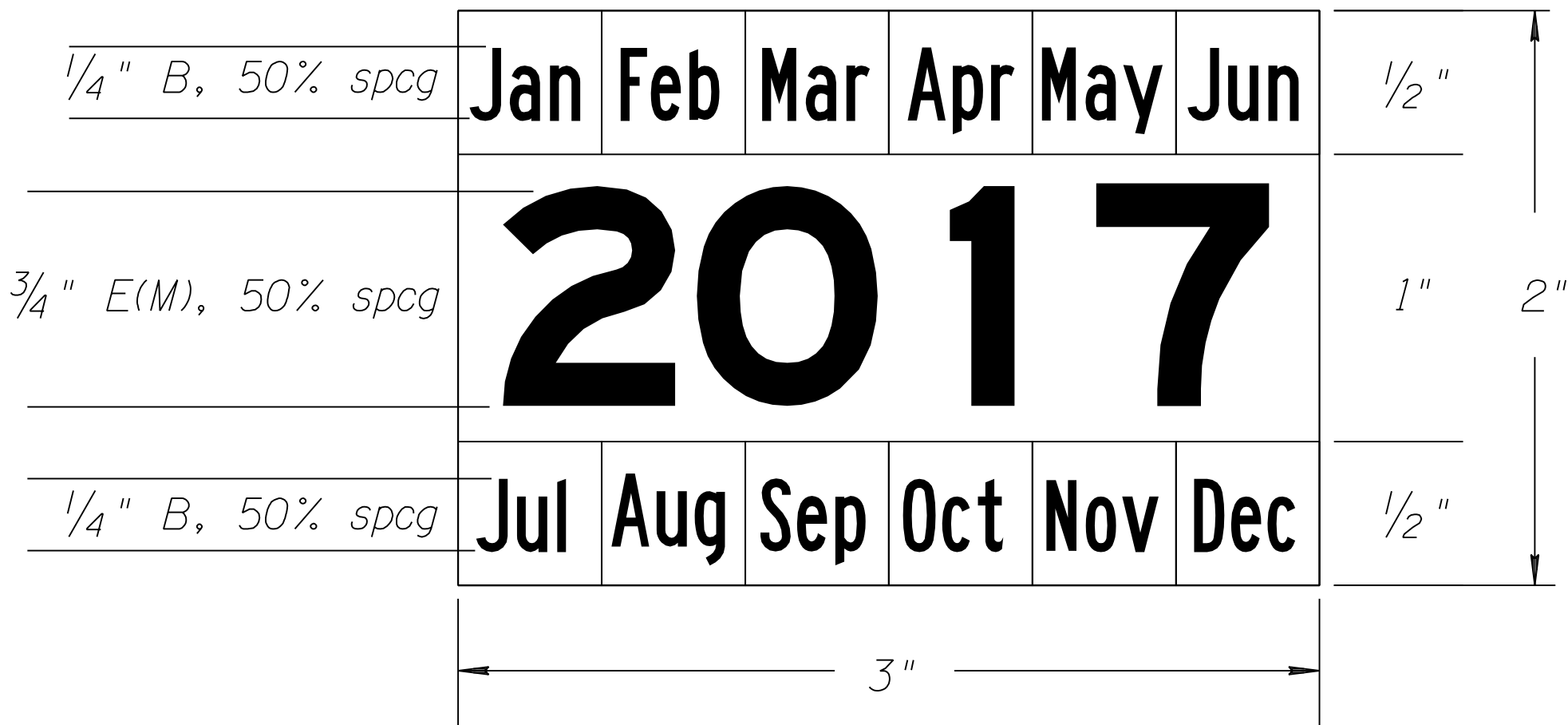
INSTALLATION DATE DECAL
