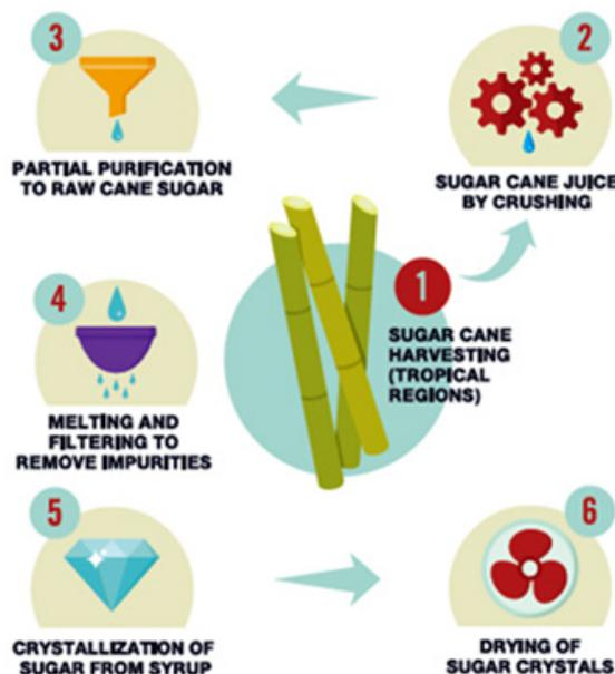
Figure 1: Sugarcane refining process
