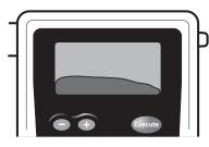
As the subject blows into the mouthpiece, the FC10 will show a graph of the breath flow on the display, as well as showing the amount of liters. Liters are shown in the upper left corner.
