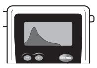
If the FC10 detects alcohol, the alcohol level is graphed and will be displayed before the result.
