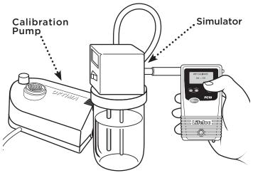
Verify the "CAL STANDARD" is set to the concentration of certified alcohol solution you will be using when you calibrate. To select new Calibration Standard, see page 16.
