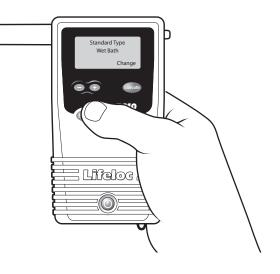
Press the **Function** button to save settings. Momentarily press **Power** to return to the testing mode.
