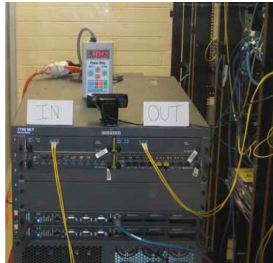
Figure 14. Experimental setup to validate the router power consumption model
