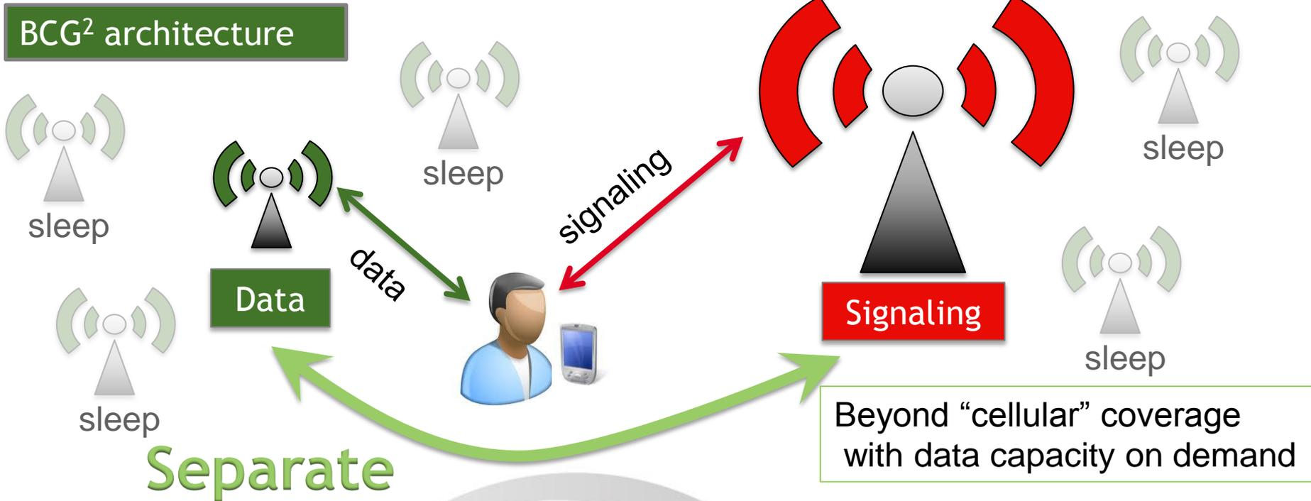
Separation of signaling and data functions at the radio interface:
