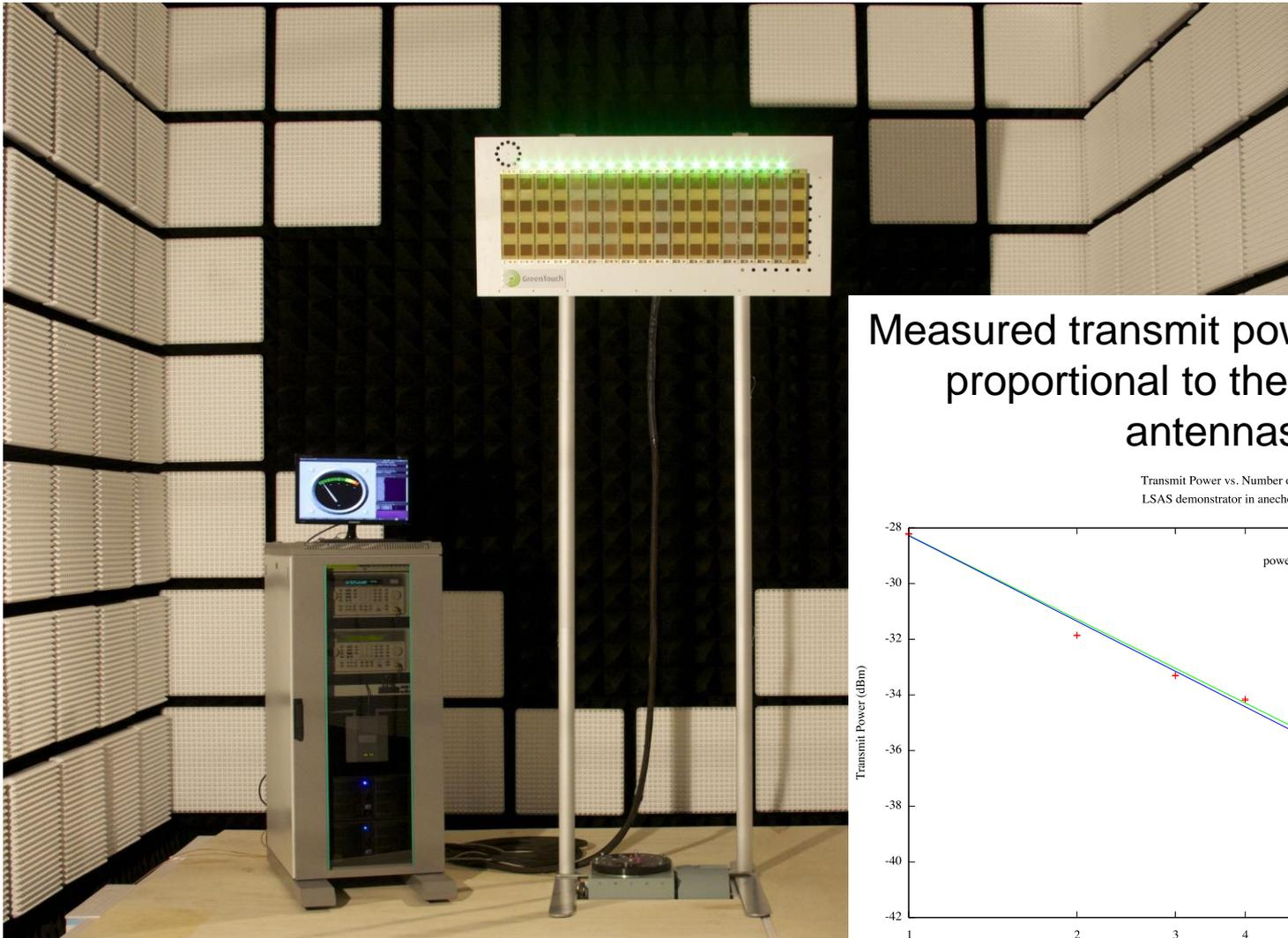
Measured transmit power is inversely proportional to the number of antennas:
