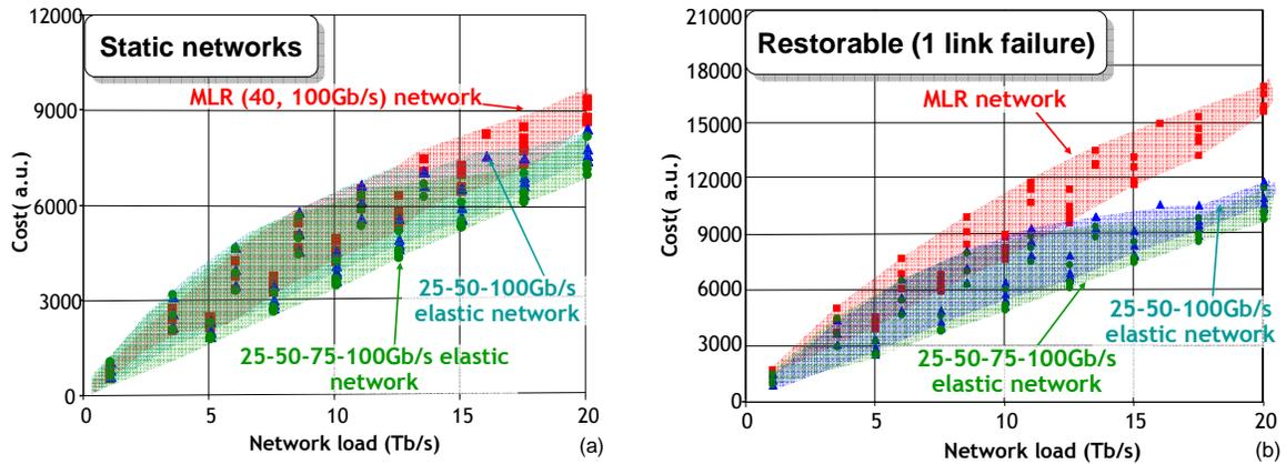
Figure 4: Cost comparison between fixed and elastic datarate networks for static (a) and restorable (b) network dimensioning.
