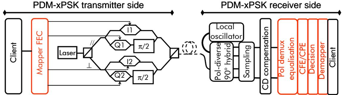
**Figure 1:** Example of a versatile PDM-xPSK transponder architecture. Left-hand side: transmitter, right-hand side: receiver. The red boxes indicate the parts of the transmitter and receiver sides that require a redesign compared to the legacy 100 Gb/s PDM-QPSK transponder architecture.
