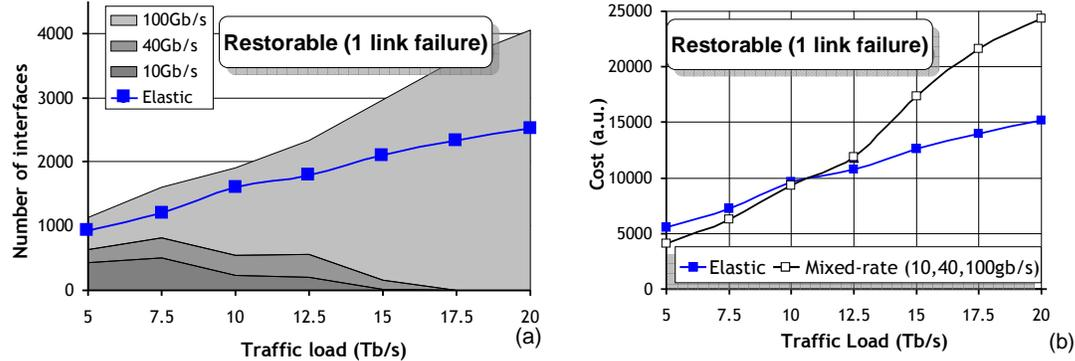
**Figure 3:** Number of interfaces required for the mixed-rate and elastic networks (a) and whole cost of the two network scenarios (b) as a function of the transported traffic load, the dimensioning is performed such as the network is resilient for one link failure.
