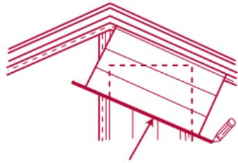
Use a piece of siding, draw line here to reflect angle of roof onto siding
