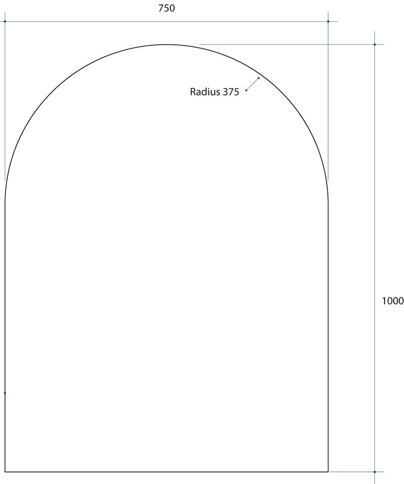
Note: All dimensions are in millimetres (mm)
