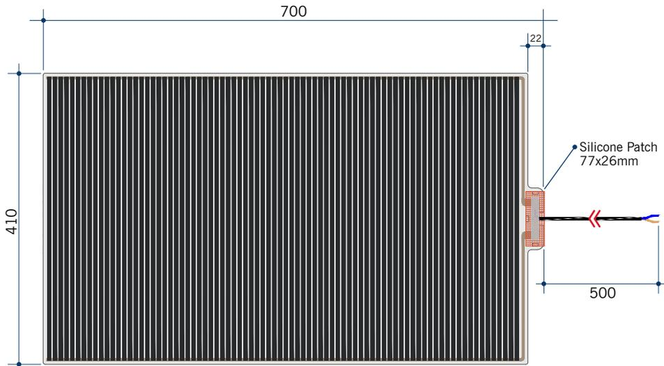
Note: All dimensions are in millimetres (mm)
