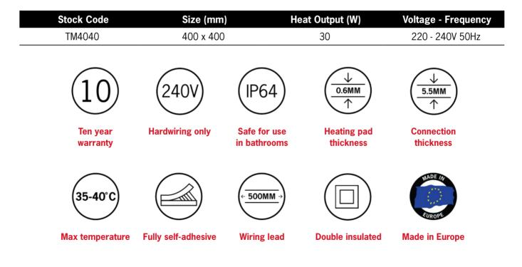
Thermomirror demisters must be installed by a qualified electrican. The demister cannot be cut, pierced or modified in anyway.
