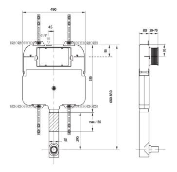
The slim concealed, dual flush cistern is made from high density polyethylene, incorporating inbuilt overflow. Due to it's slim design, the cistern can be installed in a standard 90mm metal or timber stud wall application.
