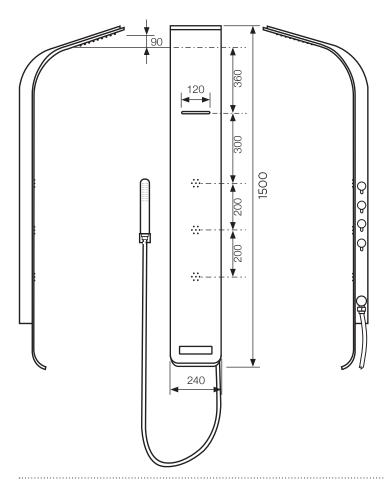
The Synergii shower panel is created from aluminum alloy with durable stainless steel hoses and brass bodies for the body jets.
