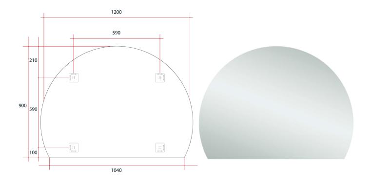
Note: All dimensions are in millimetres (mm)
