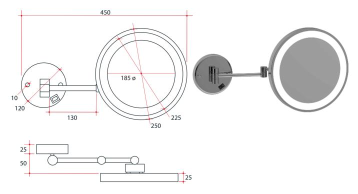
Note: All dimensions are in millimetres (mm)
