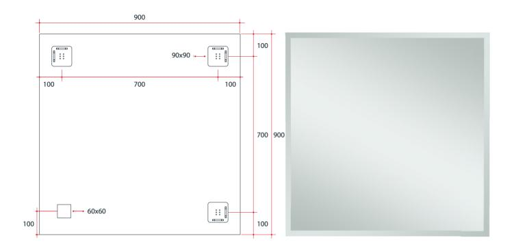
Note: All dimensions are in millimetres (mm)
