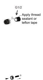
2. Screw the adapter onto the outlet. Push wall plug into drilled hole. Fit lower mounting pillar in place with screw. Tighten firmly.
