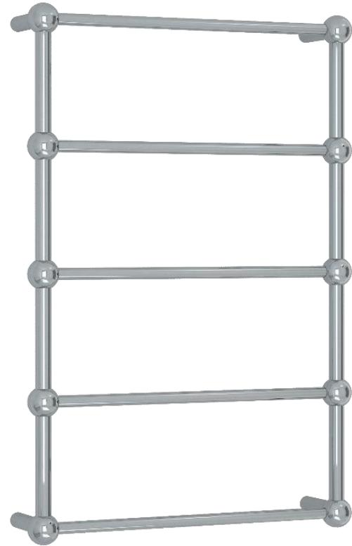
This rail has Multiflex wiring which means that there is a connection point on both the left and right hand side of the rail and the lead can be connected to either side. Being a dry electric element rail, this can be mounted either way up meaning the wiring can be from any of the four mounting points.
