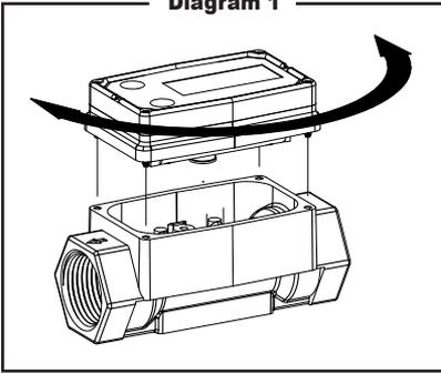
Avoid electronically “noisy” environments. Install at least 6 inches (15.2 cm) away from motors, relays, or transformers.
