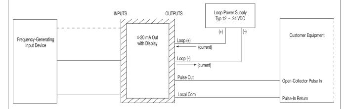
NOTE 1: Loop power supply electrically isolated
