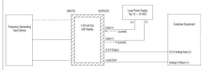
NOTE 1: Loop power supply electrically isolated from customer equipment
