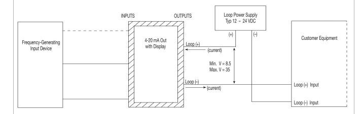
NOTE: Minimum loop power supply voltage required: 8.5V + (Max - Customer - Equipment - Drop) + (Wiring - IR - Drop) CAUTION:
