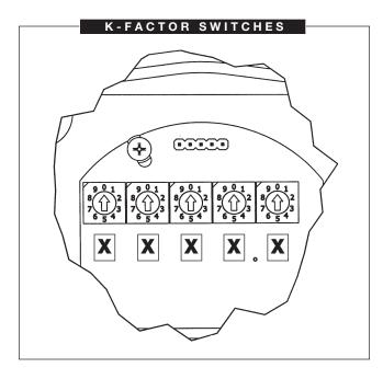
The "X" markers represent the digits of the K-factor. This allows a K-factor range of 0000.1 to 9999.9. The switches are arranged and labeled as follows:
