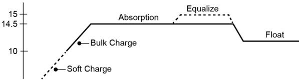
**Auto Equalize:** The GP-PWM-30-SQ has an automatic equalize feature that will charge and recondition your batteries once a month at a higher voltage to ensure that any excess sulfation is
