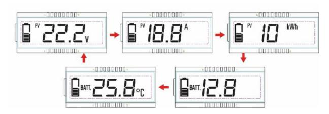
Display: PV voltage, PV current, PV power, Battery voltage and Battery temperature
