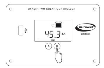
Push the **B Button** to show the number of amp hours charged since the last reset.
