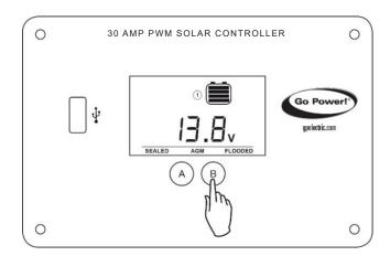
To select the battery charging profile, press and hold the **B Button**. This will cause the current battery type to flash.
