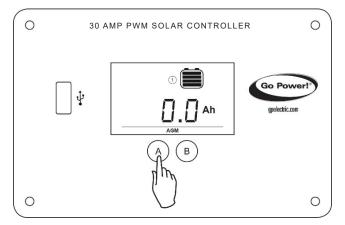
To reset the count of ampere hours charged, toggle to the ampere hours charged. Press and hold the **A Button** for 6 seconds to reset the counter to zero.
