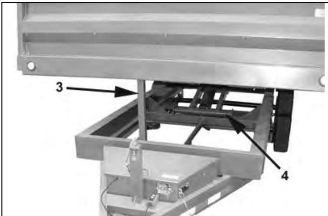
Support Body and Lubricate Cylinder Ends – Figure 8-3
