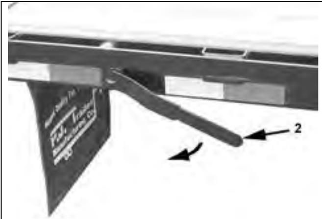
Dovetail Mechanical Stop Handle – Figure 6-3
