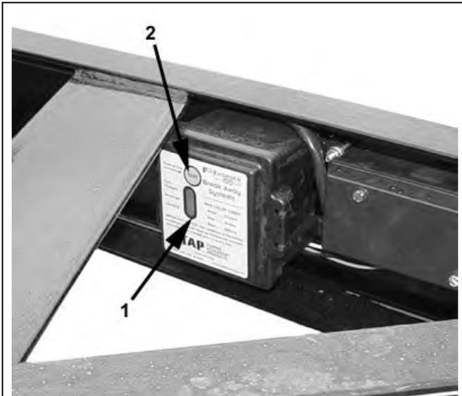
Breakaway Brake Battery Charger – Figure 4-9
