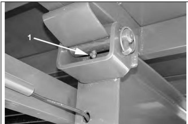
Lubricate Dump Body Pivot Hinges – Figure 8-1
