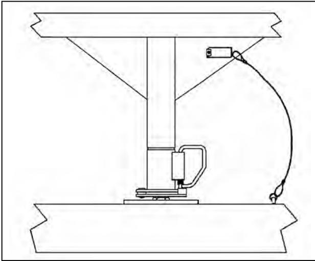
Breakaway Brake Lanyard – Figure 4-10.
