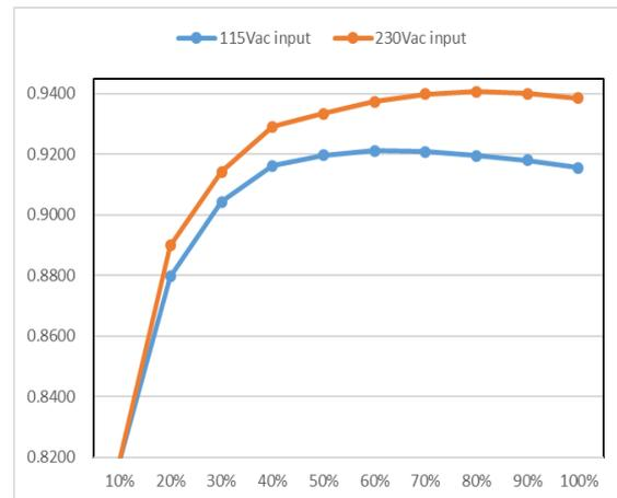
Figure 1-1. Typical efficiency Curve for 42V (1200W max)
