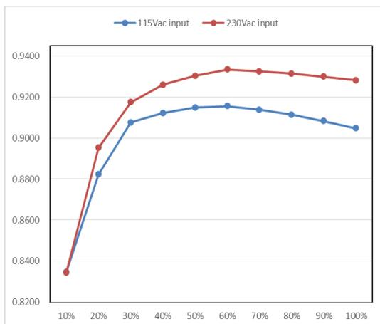
Figure 1. Typical efficiency Curve for 24V (1200W max)
