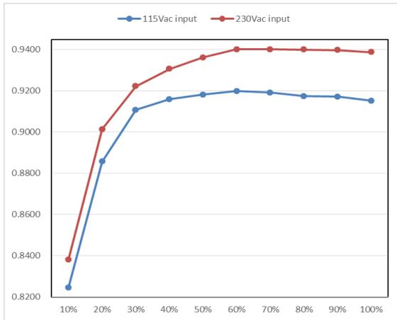
Figure 1-2. Typical efficiency Curve for 48V (1200W max)
