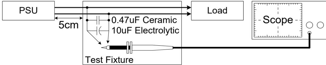
Figure 3 Ripple & Noise testing set up
