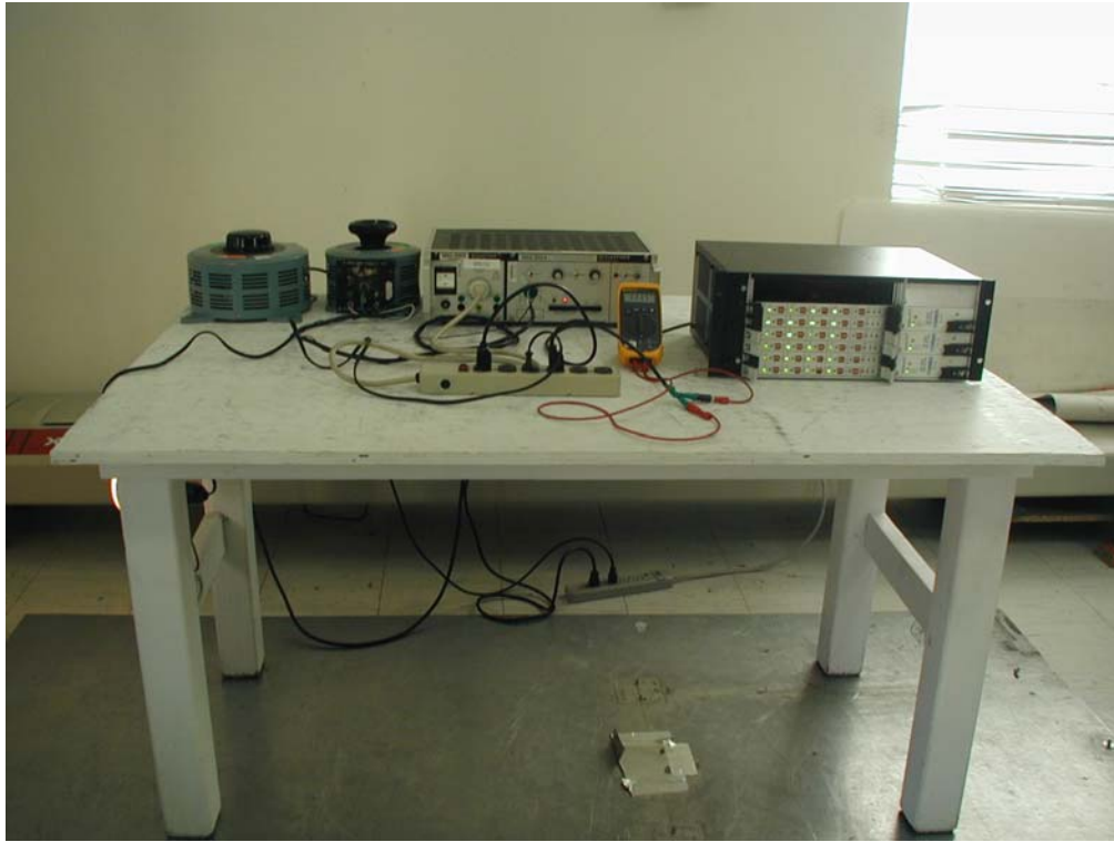
Figure 21: Voltage Dips, Short Interruptions and Voltage Variations Test Setup (S/N: 115329)
