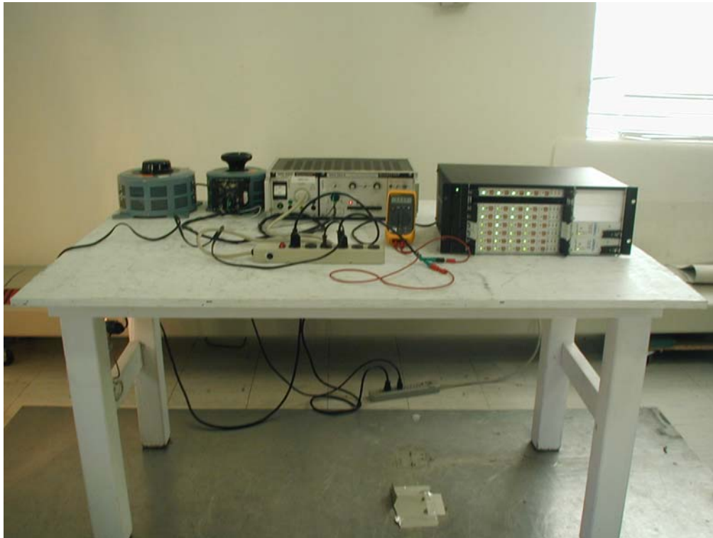
Figure 22: Voltage Dips, Short Interruptions and Voltage Variations Test Setup (S/N: 106665)
