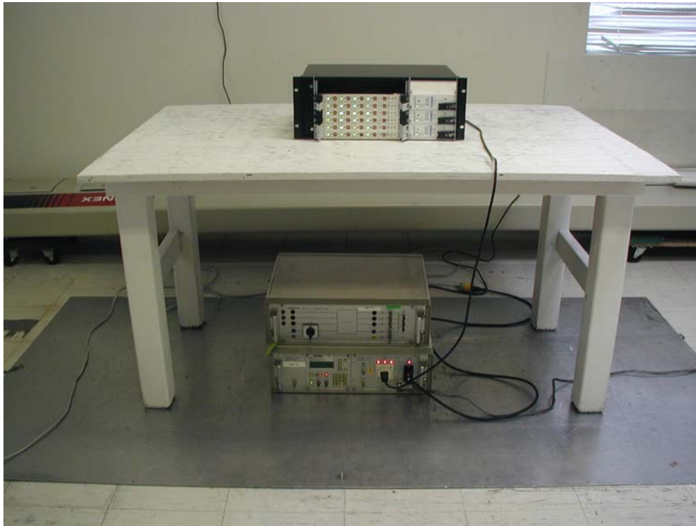
Figure 15: Electrical Fast Transients/Burst Test Setup (S/N: 115329)
