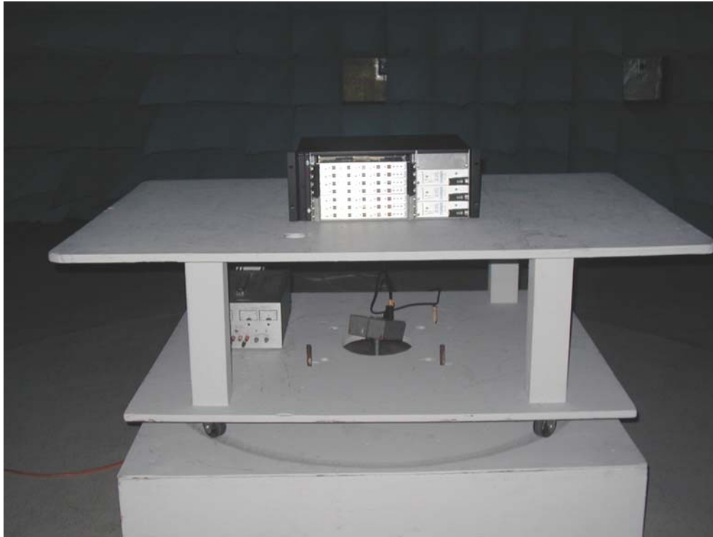
Figure 7: Front View: Chamber Radiated Maximized Emissions (S/N: 106665)
