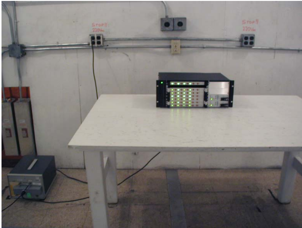
Figure 3: Front View, Power Line Conducted Maximized Emissions (S/N: 106665)
