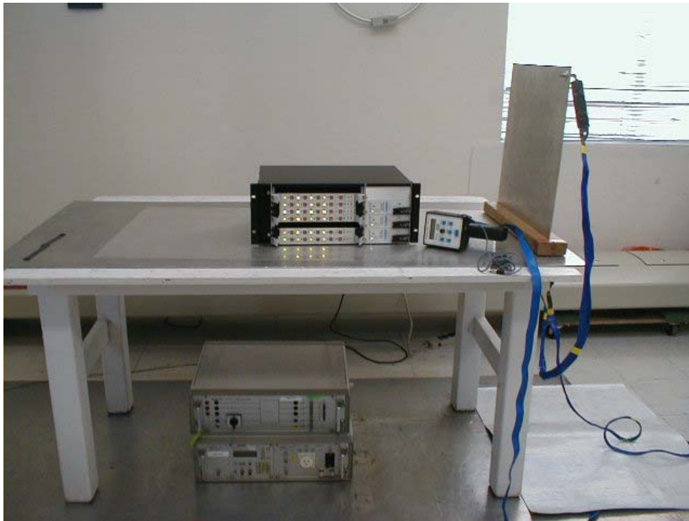
Figure 13: ESD Test Setup (S/N: 115329)
