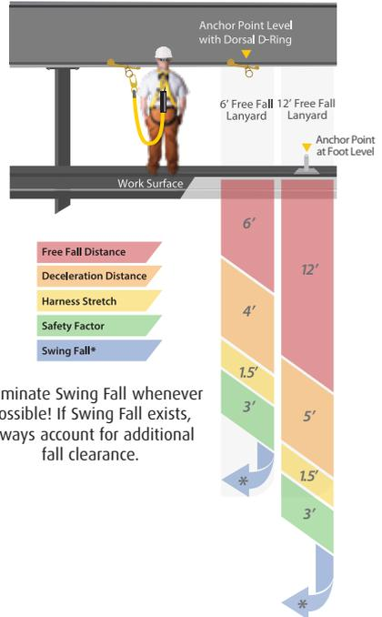
\*Eliminate Swing Fall whenever possible! If Swing Fall exists, always account for additional fall clearance.
