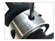
5 Tighten one of the 1/4-28 set screws until tight. Note: This will intentionally offset the Bar Clamp, Then tighten the second 1/4-28 set screw. When completed it is normal for the bar clamp to be offset from the shaft. **NOTE:** The rubber flange will be pierced for the set screws to mate with the tool.
