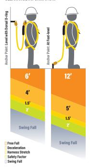
WARNING! Eliminate Swing Fall whenever possible! If swing fall exists, always account for additional fall clearance.
