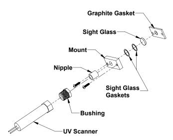
Figure 32: UV Scanner Assembly
