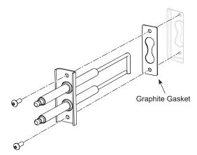
Figure 30: Igniter Electrode Assembly
