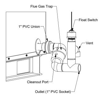
Figure 11: Condensate Trap Assembly
