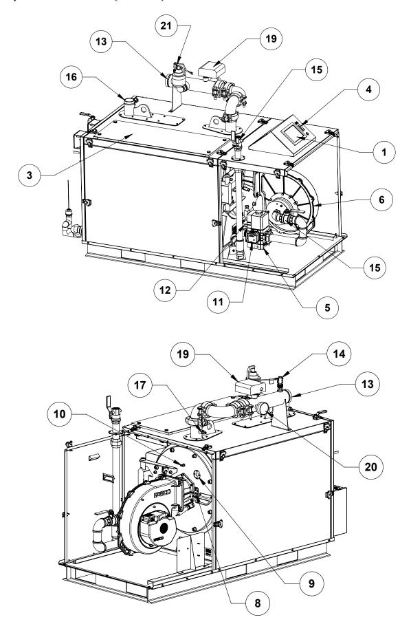
Figure 2: Component Identification
