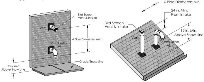
Figure 6: Horizontal Sidewall Termination
