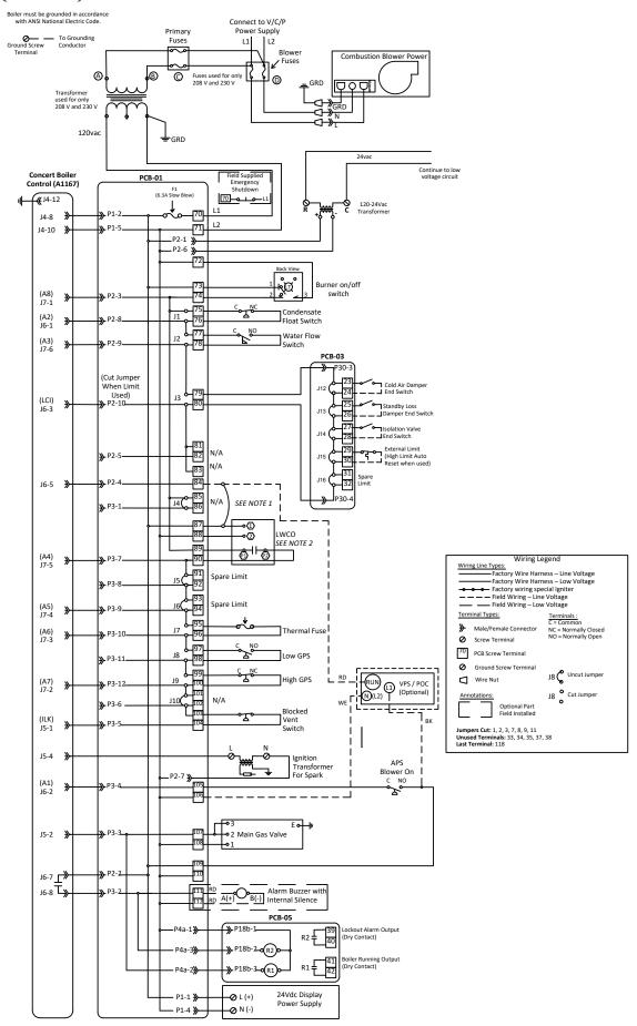
Figure 26: Single Phase Wire Diagram
