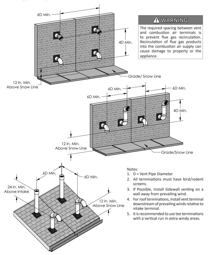
Figure 9: Multiple Appliance Direct Vent Termination
