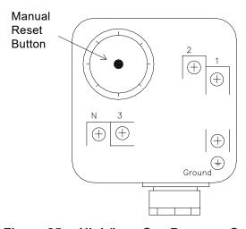
Figure 25: High/Low Gas Pressure Switch
