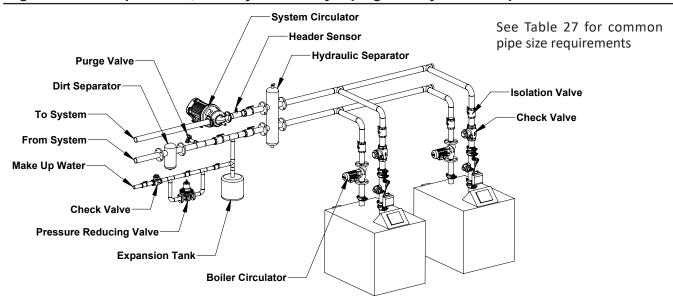
Figure 18: Single Boiler with Indirect Domestic Hot Water Heating
