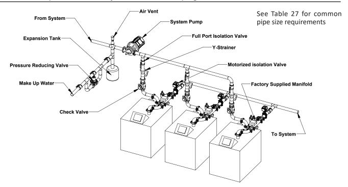
Figure 16: Single Boiler, Variable Primary Piping
