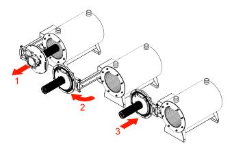
Figure 33: Burner Door Opening
