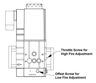
Figure 29: Gas Valve Air/Fuel Adjustment
