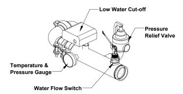
Figure 12: Factory Supplied Water Manifold
