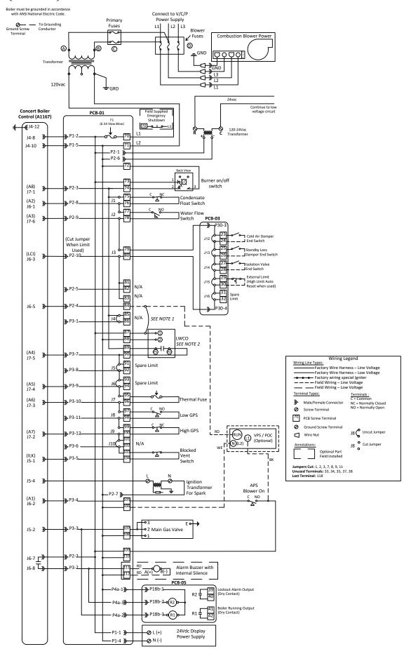
Figure 27: Three Phase Wire Diagram
