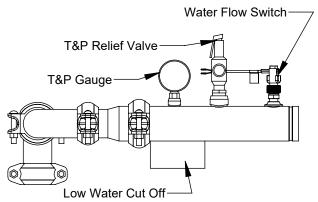
Figure 19: Hot Water Outlet Manifold (W)
