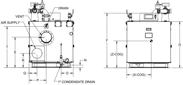
Figure 1: Boiler Dimensions
