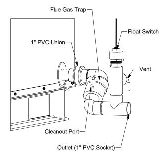
Figure 11: Condensate Trap Assembly
