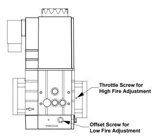
Figure 22: Gas Valve Air-to-Fuel Adjustment
