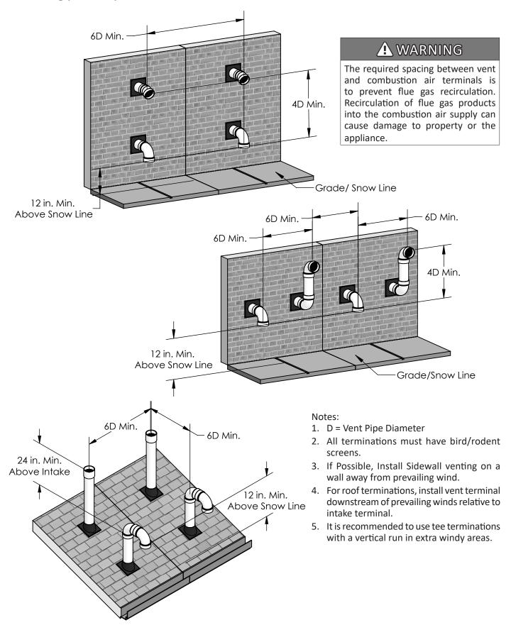
Figure 9: Multiple Appliance Direct Vent Termination
