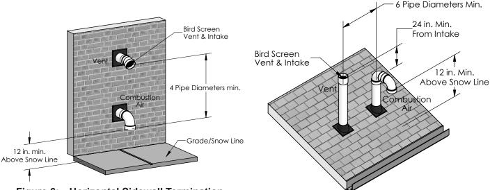
Figure 6: Horizontal Sidewall Termination
