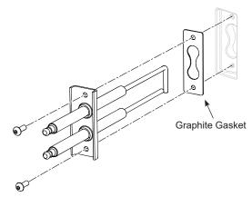
Figure 23: Igniter Electrode Assembly
