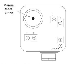
Figure 18: High/Low Gas Pressure Switch
