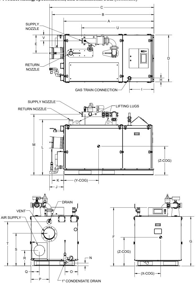
Figure 1: water heater dimensions
