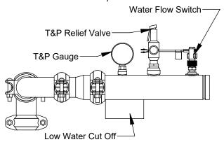
Figure 12: Hot Water Outlet Manifold
