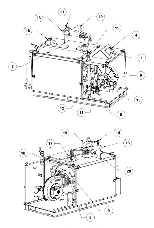
Figure 2: Component Identification
