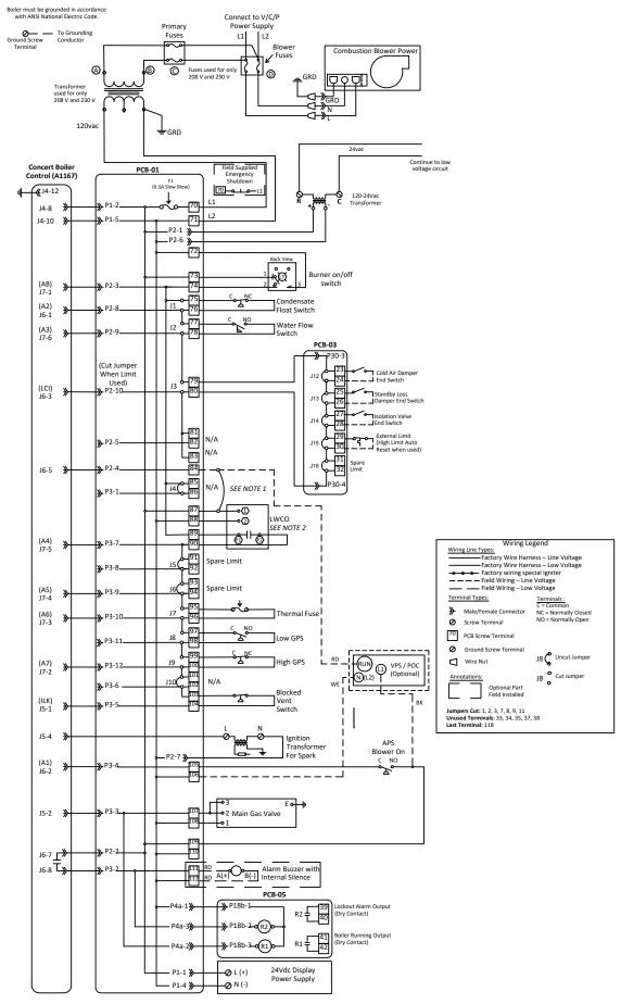
Figure 19: Single Phase Wire Diagram
