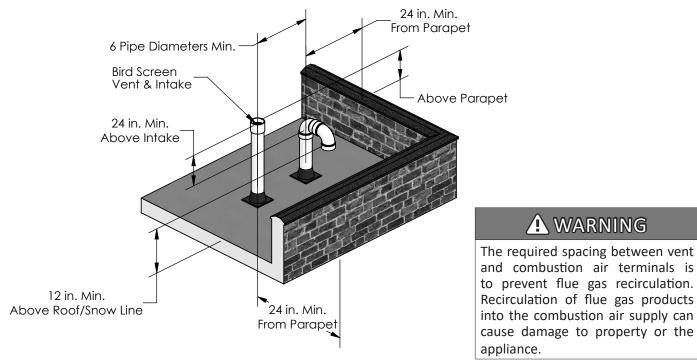
Figure 8: Flat Roof Vent Terminations
