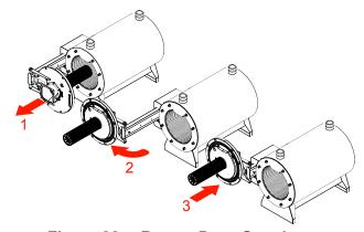
Figure 26: Burner Door Opening
