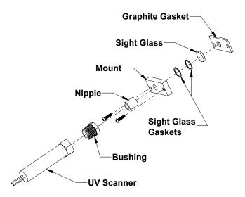
Figure 25: UV Scanner Assembly
