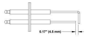
Figure 25: Igniter Electrode Gap
