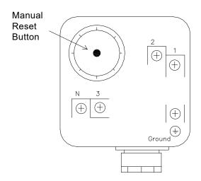
Figure 19: High/Low Gas Pressure Switch
