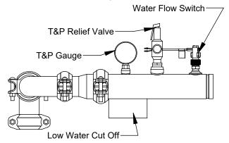
Figure 12: Hot Water Outlet Manifold
