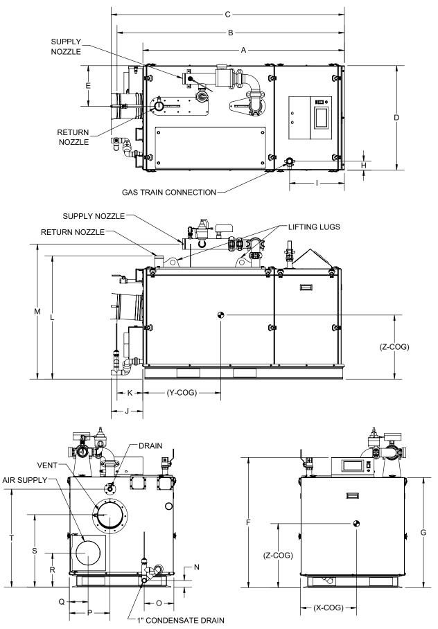
Figure 1: Citadel water heater dimensions
