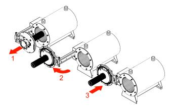
Figure 27: Burner Door Opening
