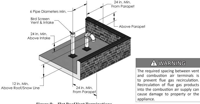
Figure 8: Flat Roof Vent Terminations
