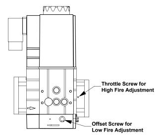
Figure 23: Gas Valve Air-to-Fuel Adjustment
