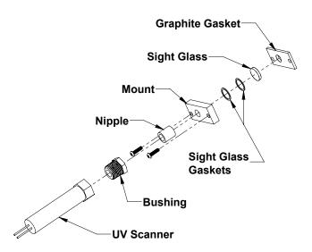
Figure 26: UV Scanner Assembly
