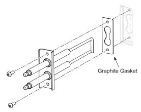
Figure 24: Igniter Electrode Assembly
