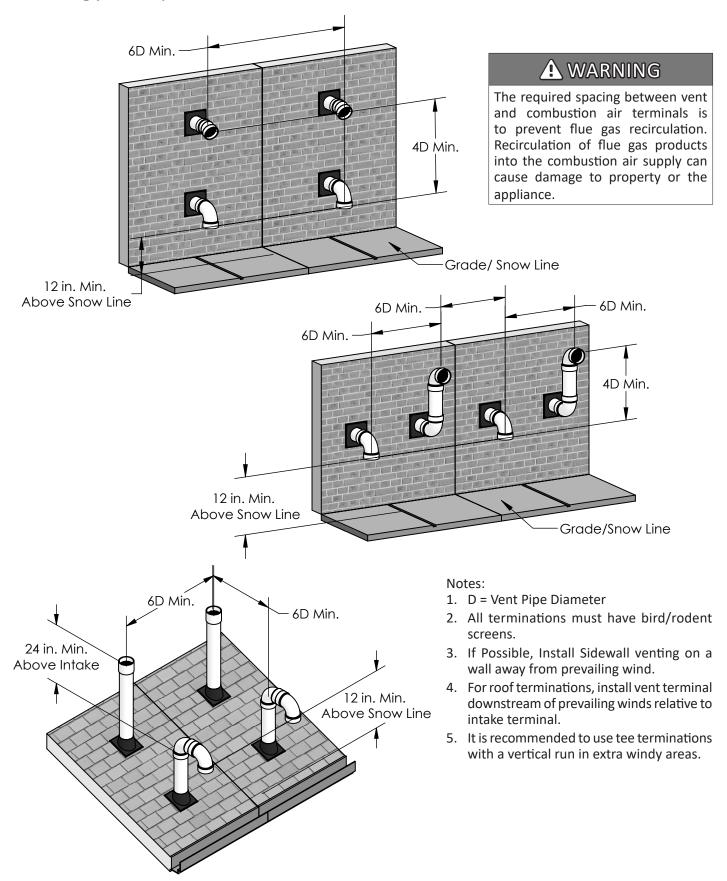
Figure 9: Multiple Appliance Direct Vent Termination
