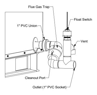
Figure 11: Condensate Trap Assembly
