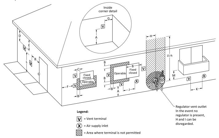
Figure 5: Vent Terminal Clearances
