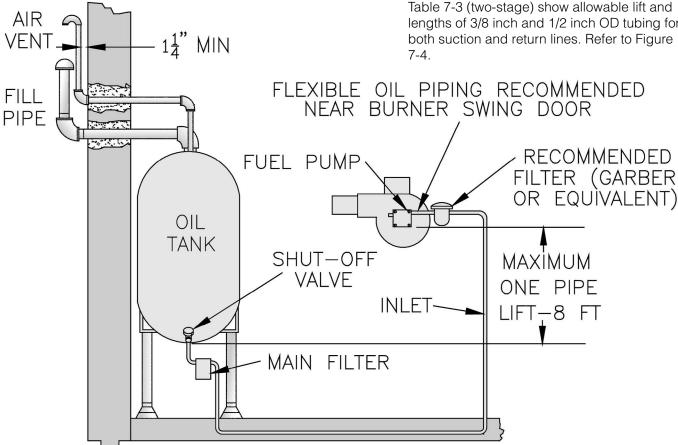
Figure 7-1: Single-Pipe Installation
