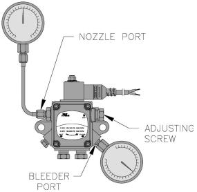
Figure 8-1: Adjusting Fuel Pump Pressure
