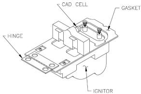
Figure 8-3: Cad Cell Location
