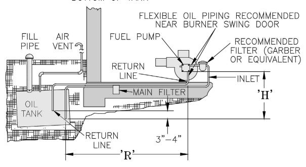
Figure 7-4: Two-Pipe Installation
