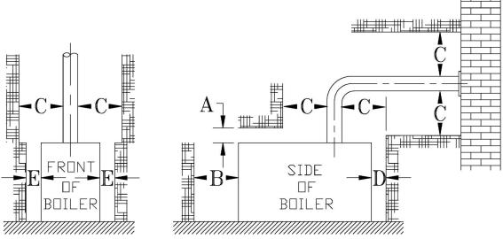
Figure 2-1: Minimum Installation Clearances to Combustible Materials (Inches)
