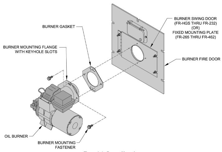
Figure 3-4: Burner Mounting
