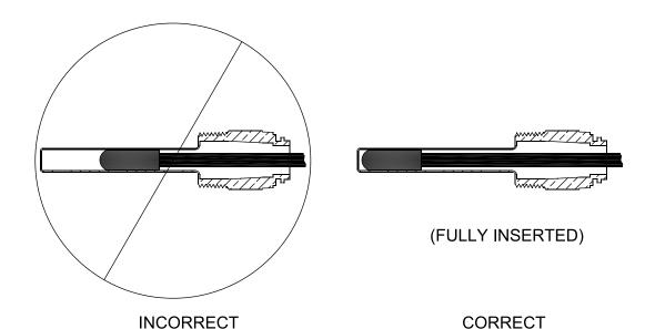
Figure 3-1: Limit Sensor Insertion
