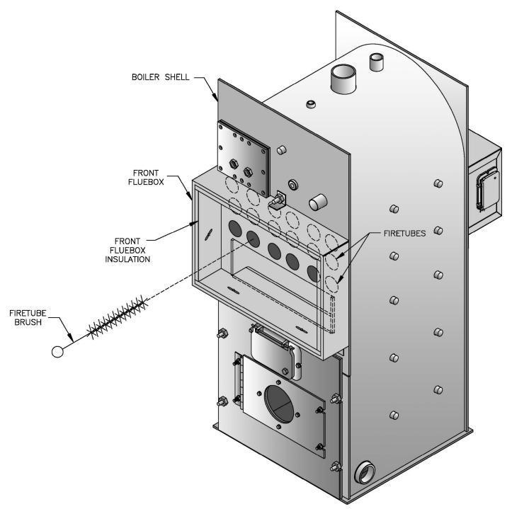
Figure 11-1: Cleaning of FR Boiler
