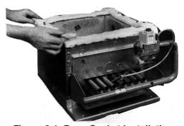
Figure 6-1: Base Gasket Installation
