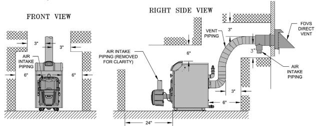
Figure 1-5: Direct Vent Boiler - Minimum Installation Clearances To Combustible Materials (Inches)
