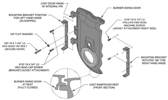
Figure 2-2: Partial Front View - Burner Swing Door Mounted to Boiler - Fully Closed and Secured
