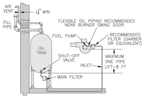
Figure 7-1: Single Pipe Oil Line
