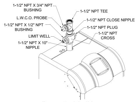
Figure 3-4: Near Boiler Piping
