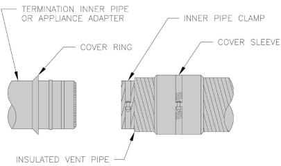
Figure 5-9: Vent Pipe Assembly to Vent Termination Inner Pipe and Appliance Adapter
