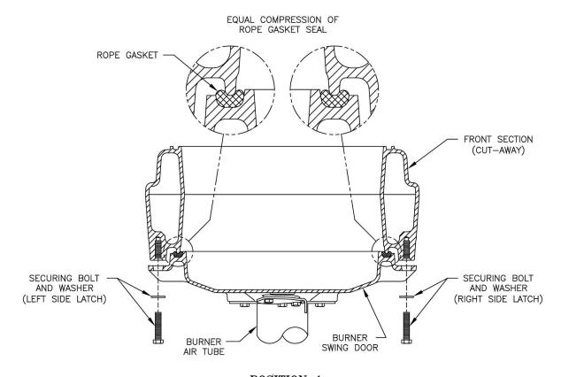
POSITION 1 (PROPERLY CLOSED AND SECURED)
