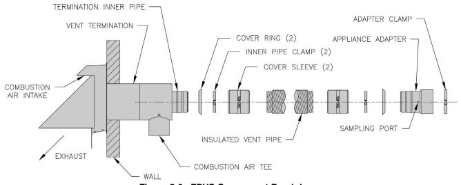
Figure 5-6: FDVS Component Breakdown
