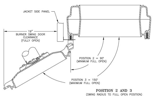
Figure 2-3: Top View - Burner Swing Door Mounted to Cast Iron Block Assembly (Jacket Removed for Clarity)
