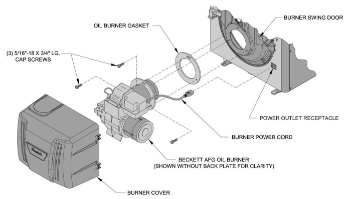
Figure 2-11: Oil Burner Installation (Beckett shown)
