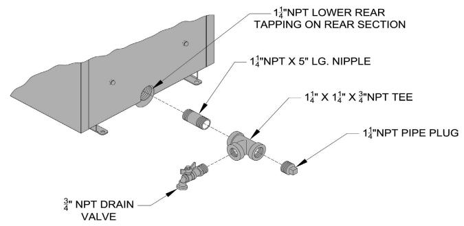
Figure 2-7: Piping Arrangement for Drain Valve and Indirect Water Heating Return
