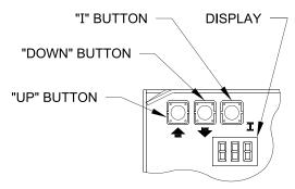
Figure 9-3: Boiler Control Key Function & Orientation
