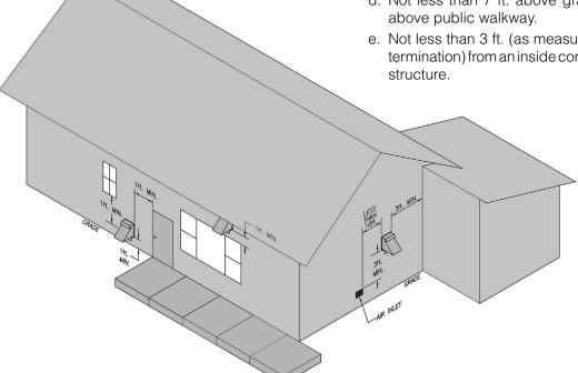
Figure 5-1: Vent Terminal Location
