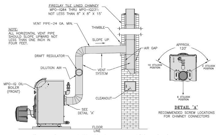
Figure 4-1: Recommended Vent Pipe Arrangement and Chimney Requirements
