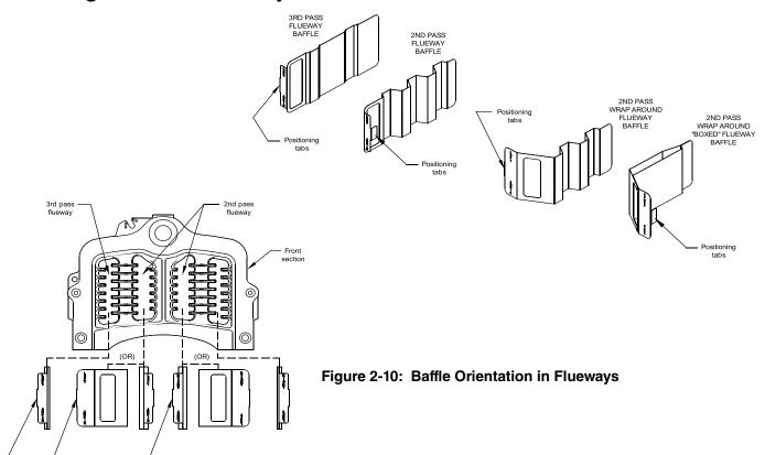
**Step a.** Install stainless steel baffles provided in miscellaneous parts carton as follows, refer to Table 2-1 and Figure 2-10:
