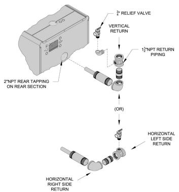
Figure 2-6: Return Injector Piping and Relief Valve Assembly Details
