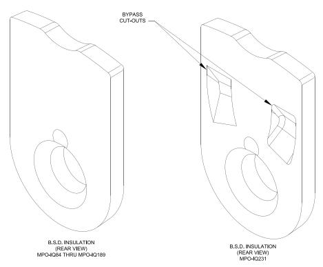
Figure 2-5: Burner Swing Door Insulation
