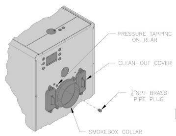
Figure 4-3: Smokebox Pressure Tapping for Checking Draft at Breech
