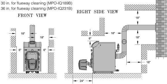
Figure 1-4: Chimney Vented Boiler - Minimum Installation Clearances To Combustible Materials (Inches)
