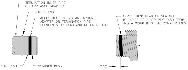
Figure 5-10: Vent Pipe Ends, Vent Termination and Appliance Adapter Sealing
