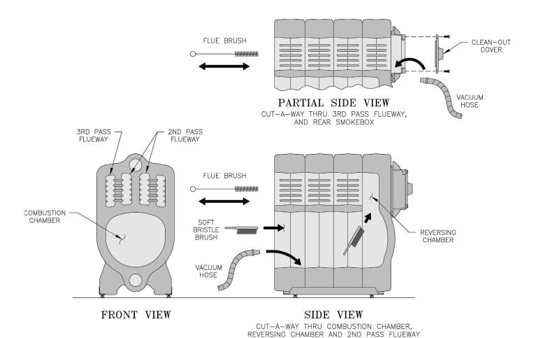
Figure 11-1: Cleaning of Boiler Flueways
