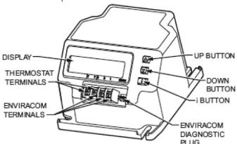
Figure 8-1: R7284 Oil Primary Terminals, Display and Function Buttons
