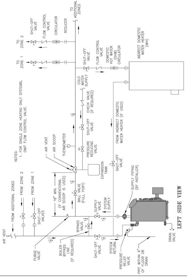
Figure 3-2: Recommended Water Piping for Circulator Zoned Heating Systems
