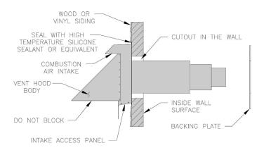
Figure 5-4: Vent Hood Body Installation
