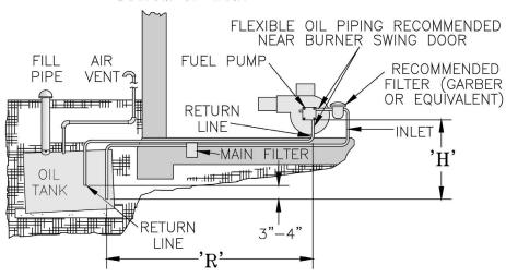
Figure 7-4: Two Pipe Oil Lines
