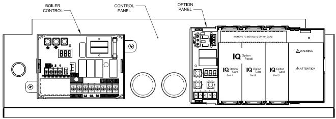
Figure 9-1: Boiler Control & Option Panel Orientation
