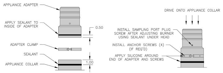
Figure 5-8: Appliance Adapter Installation
