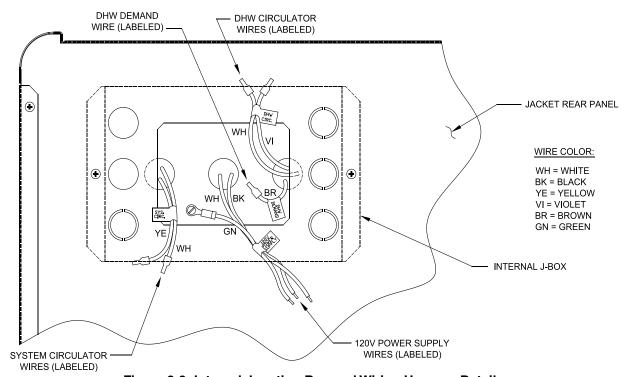
Figure 2-9: Internal Junction Box and Wiring Harness Details
