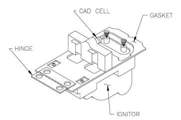
Figure 8-2: Cad Cell Location
