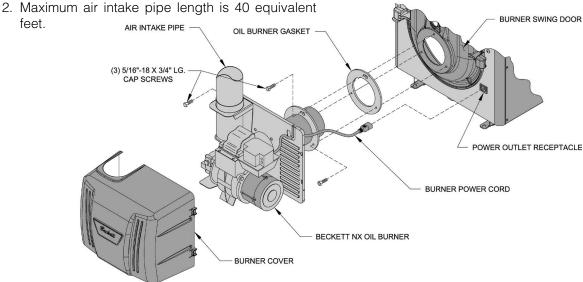
Figure 5-12: Oil Burner Installation (Beckett shown)
