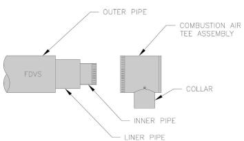
Figure 5-5: Combustion Air Tee Assembly Installation
