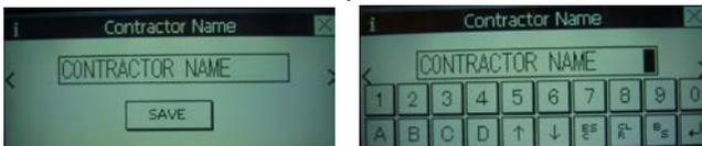
Press “Contractor Name” display to open a keypad. After entering contractor info, press the “SAVE” button to store the content.
