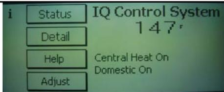
The Home Screen provides supply water temperature, central heat and domestic hot water (DHW) heat demand status as well as “Energy Save” status. Energy Save On appears when the Reset Setpoint is reduced below the HL Setpoint.
