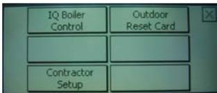
The Adjust Mode Menu screen allows the technician to choose the IQ Control System component to adjust by simply selecting the item.
