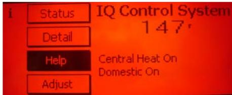
(Screen shows faulted sensor)
